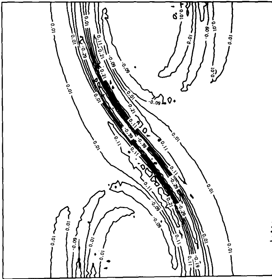
FIG. 3. Current sheets are formed by the twisting and stretching of the magnetic field in Fig. 2. The current is especially intense in the center, and there the magnetic diffusion and reconnection are occurring at an accelerated rate.
